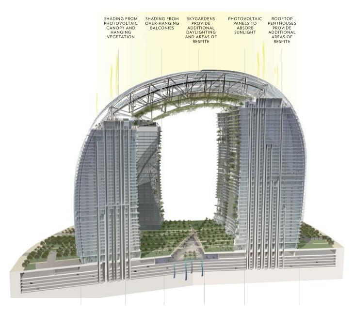
PUBLIC AREAS IN THE TOWERS ARE NATURALLY FILTERED BY VEGETATED WALLS SALT WATER TOLERANT LANDSCAPE FOR LOWER LEVEL SHADING PLAZA AND RETAIL AREAS ARE PASSIVELY COOLED BY THE EARTH AND ADDITIONAL SHADING CONNECTIONS
